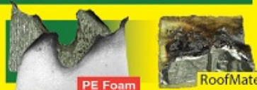
Dripping observed in burning PE Foam contributes to spread of fire
