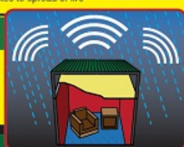
Dripping observed in burning PE Foam contributes to spread of fire
